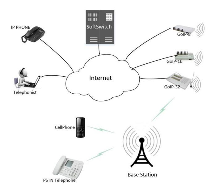
**VoIP GSM Gateway GoIP-32** HyberTone's GoIP-32 is a VoIP GSM Gateway for call termination (VoIP to GSM) and origination (GSM to VoIP). It is SIP&H.323 based and compatible with Asterisk, Trixbox, 3CX, SIP Proxy Server, VoipBuster. It can enable to make 32 calls simultaneously from IP phones to GSM networks and GSM networks to IP phone.
