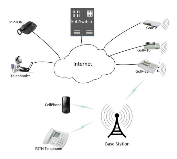
**VoIP GSM Gateway GoIP-16** HyberTone's GoIP-16 is a VoIP GSM Gateway for call termination (VoIP to GSM) and origination (GSM to VoIP). It is SIP&H.323 based and compatible with Asterisk, Trixbox, 3CX, SIP Proxy Server, VoipBuster. It can enable to make 16 calls simultaneously from IP phones to GSM networks and GSM networks to IP phone.
