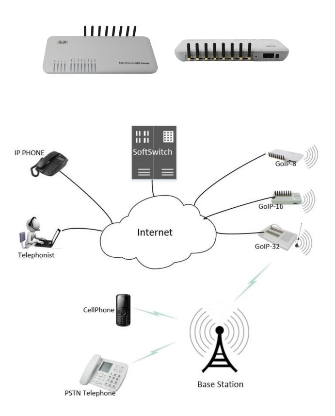
**VoIP GSM Gateway GoIP-8** HyberTone' GoIP-8 is a VoIP GSM Gateway for call termination (VoIP to GSM) and origination (GSM to VoIP). It is SIP&H.323 based and compatible with Asterisk, Trixbox, 3CX, SIP Proxy Server, VoipBuster. It can enable to make 8 calls simultaneously from IP phones to GSM networks and GSM networks to IP phone.
