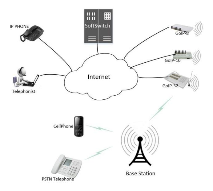
**VoIP GSM Gateway GoIP-4** HyberTone's GoIP-4 is a VoIP GSM Gateway for call termination (VoIP to GSM) and origination (GSM to VoIP). It is SIP&H.323 based and compatible with Asterisk, Trixbox, 3CX, SIP Proxy Server, VoipBuster. It can enable to make 4 calls simultaneously from IP phones to GSM networks and GSM networks to IP phone.
