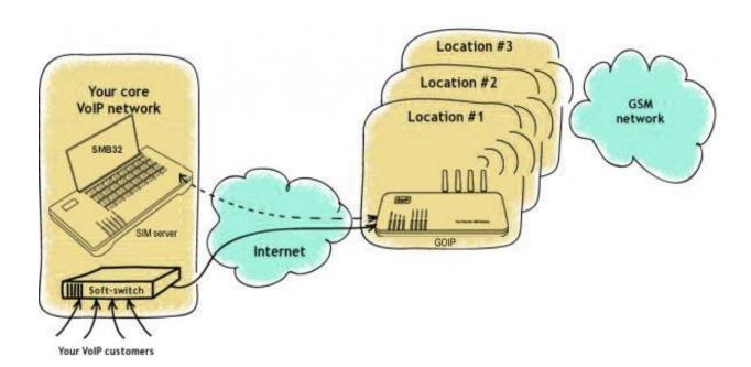
**Remote SIM Bank SMB32** is a device that holds 32 SIM cards that can be accessible remotely. So there will be a virtual SIM card placed on your GSM gateway at anytime you want. With SIM bank you can use all your SIM cards in one location (usually your core network) and manage easily.
