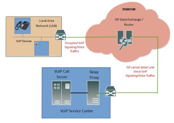
2. Relay Proxy solves the NAT issue by re-routing data traffics from VoIP devices to the VoIP Call Server and vice versa as shown in the diagram below. All data packets now have the proper destination IP, so that they can be delivered. In general, if SIP registration is not successful or one way audio occurs when a call is established, you can try to solve the problems with Relay Proxy.
