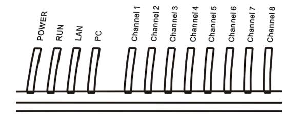
LED indicators (shown above for GoIP-8) are used to show the current status of the device. They are often used to determine if the device is working normally or not.
