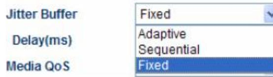
Use to designate Jitter delay buffer algorithm model. Adaptive mode is the best, other modes are used for test, please do not use in the practical action.
